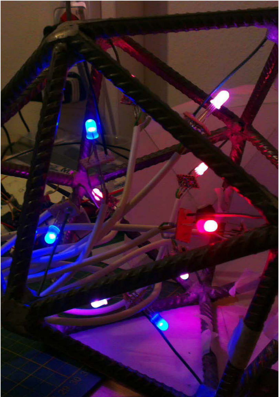
Figure 11: Successful test of lighting every LED up in an individual colour.
